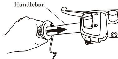
Depending on the diameter of handlebar, mounting heated grips might be very tight. Don't hit the grips by hammer, which makes them broken.
